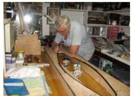
The Jig is a fixed wooden framework having all the measurements and tolerances (in compliance with the Australian EC 12 Rules as revised 2008) transcribed onto the top working surface for ease of reference. This provides the authorized builder with an accurate device to producing multiple yachts while maintaining a constant uniformity in working on these yachts.
